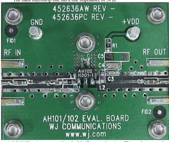
A 0  $\Omega$  0603 resistor was used on the L1 silk screen location. This can be removed from the circuit, but the placement of the C2 input shunt capacitor would have to be placed slightly further away from the device. The required electrical length of the placement is shown in the circuit configuration below.
